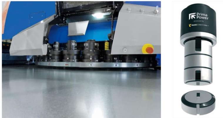
Figure 2: KONE use case measured tool holder and chosen tool
